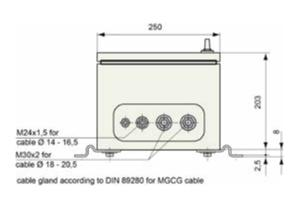
Standard control box (supply voltage 380 / 440 V - control voltage 115 / 220 V) - other voltages on request
